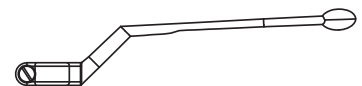
HANDLE FROM DN20 TO DN25 (without washer pos14 and screw pos15 in esplosed drawing)
